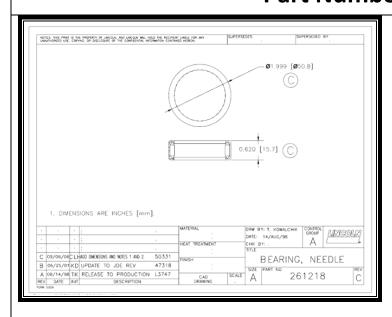
261218; Needle Bearing or Main Bearing not included in the kit 260339. Purchase this part separately. However it is pressed into the block and you need to get the old one out before you press the new one in. It can be a trying to get the old one out without damaging the block.
