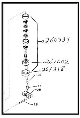
Previous components in Gear Set Kit 260339. Please note: item 261002 is no longer included in Gear Set Kit 260339. The same with main ring bearing 261218. The item 261218 was a press fit into the block and most people never used it.
