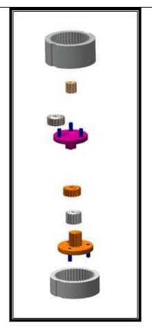
Current Arrangement of the 260339. This item was changed by Lincoln in approximately the year 2018. It is currently missing part 261002 and part number 261218 Needle Bearing. If you need these parts in your power luber, order 271892 Gear Kit assembly for the Series B 1200 Power Luber.
