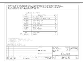
List of all the parts in the New Gear Set kit 260339. Notice missing 261218 and 261002
